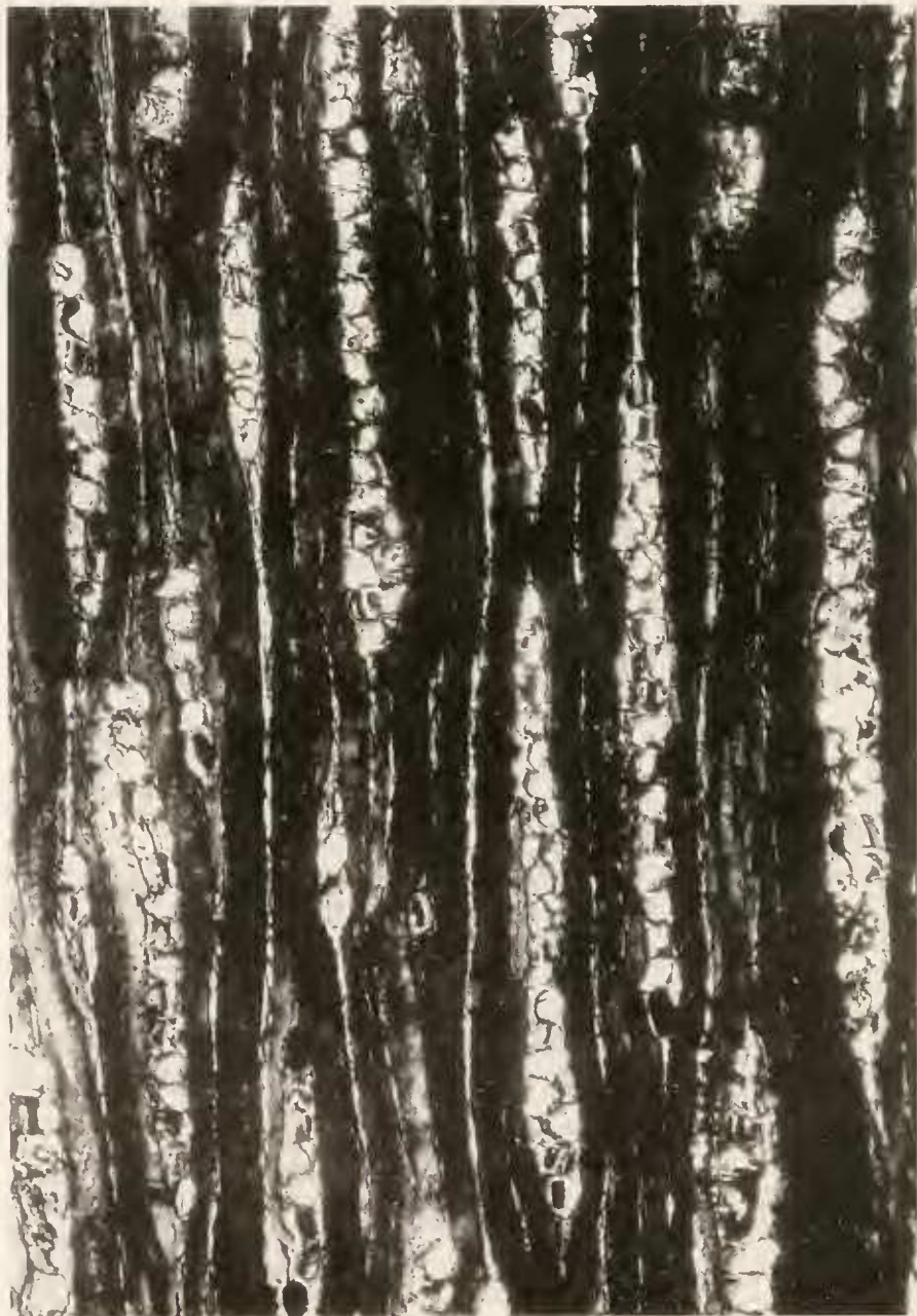
Fig. 9. Tangential longitudinal section with partly biseriate rays. x 125.
